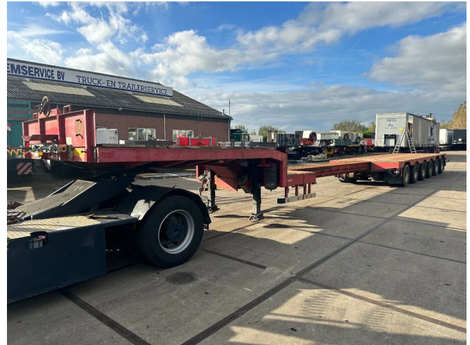
HRD 6 AXEL, 85000 KG, EXTENDABLE, LAST 2 STEERING,...
