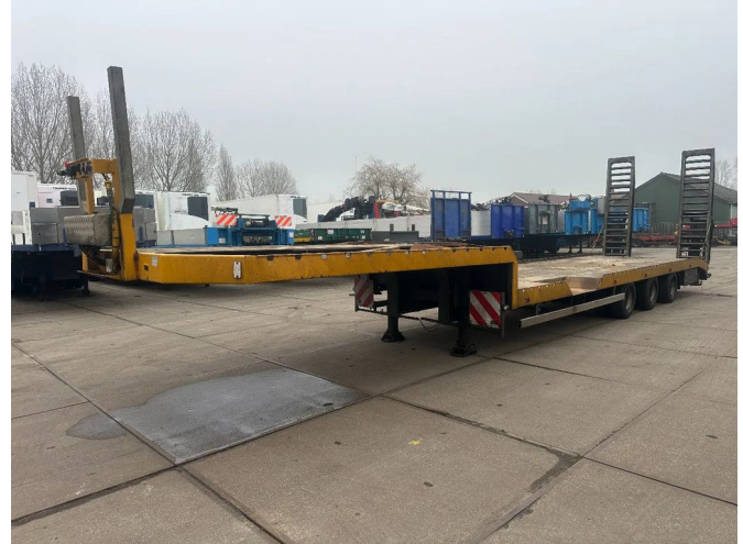
HRD 3 AXLE, HYDRAULIC RAMPS, LAST AXLE STEERING
