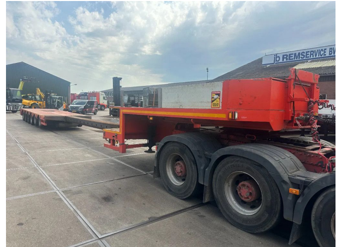
ES-GE 6 SOU-4H-1N, 6 AXLE, 4 AXLE STEERING, 2 LIFT, 8...
