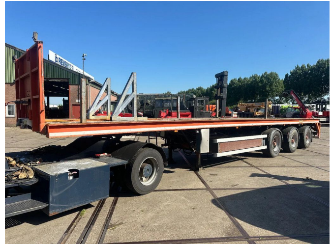
Nootboom 3 AXLE, BPW DRUM BRAKES,
