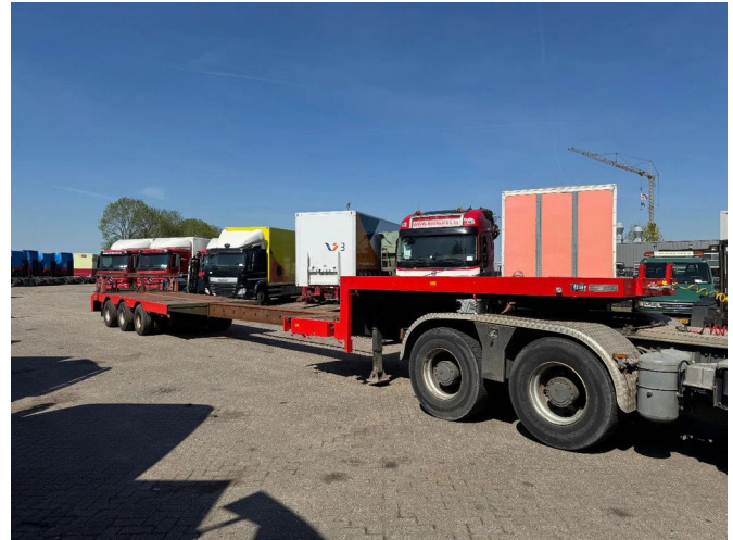
Nooteboom OSD-44-VV - 5 M EXTENDABLE + 3 AXLE SAF
