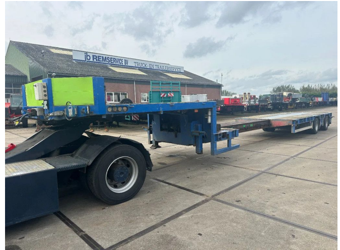
Goldhofer 2 AXLE FORCED STEERING 4,3 M EXTENDABLE
