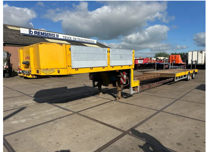
Broshuis 21N58A, 2 AXLE LAST AXLE STEERING, EXTEND...
