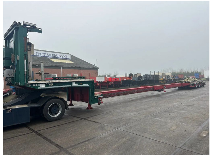
Meusburger 4 axel steering, Double extendable up to 28 mete...
